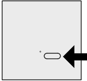
1- Press **twice** and hold down the push-button **MT** of the receiver, the buzzer will make a beep each time and then sound intermittently and slowly.
