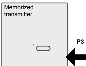
1- Press the button **P3** located inside the **already memorized transmitter**. The enabled receiver sounds continuously.
