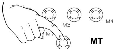
1- Press **three times** the button **MT** and hold down. The buzzer will make a beep each time and then will sound intermittently and rapidly.
