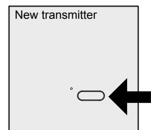
3- During the sound press the push-button of the **new transmitter** which has to be memorised; the memorization is indicated by the intermittently sound of the buzzer.
