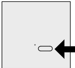
1- Press and hold down one of the push-button **M1** **o** **M2** **o** **M3** **o** **M4** of the receiver, the buzzer will make a beep each time and then sound continuously.
