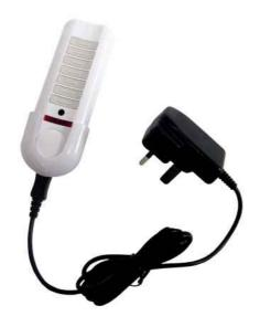
The **Wise Pod IR Interface** is used to convert the radio signal to infra-red, meaning you can use systems such as universal remotes to control your Wise Controls lighting.
