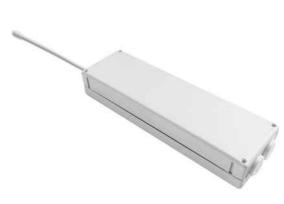
Wireless control unit for 24V rolling shutter motors for integration into the rolling shutter casing. Open-stop-close function. Input for 1 dynamic push button.
