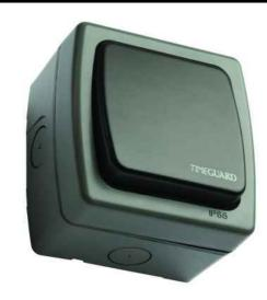
The **Weathersafe Vision Single Gang 2-Way Switch (DP)** is manufactured from tough, durable thermoplastic. It is intended for use in an outdoor environment, or one in which the protection provided by the range is required. It is rated IP66, for protection against water and dust. It will need to be fitted with waterproof cable or conduit entries to maintain their IP rating once installed.
