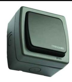
The **Weatherproof Vision Single Gang 2-Way Switch (SP)** is manufactured from tough, durable thermoplastic. It is intended for use in an outdoor environment, or one in which the protection provided by the range is required. It is rated IP66, for protection against water and dust. It will need to be fitted with waterproof cable or conduit entries to maintain their IP rating once installed.
