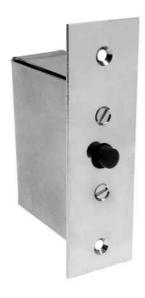
A **Door Switch** that enables you to turn a light on and off in a cupboard or room. When the door is closed on the switch the light would be turned off, as soon as the door is opened and the switch is released the light will turn on.
