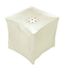
Downlighters, if not safely protected, can become a fire hazard as the hole cut in the ceiling to accommodate them compromises its fire resistance. Current building and wiring regulations have meant firehoods have become a necessity. Not only does a **Grid & Grid Trimless AR111 Firehood** seal to stop fire penetration into the ceiling void left by fittings for up to one hour, but in normal use also offer ventilation to prevent the light fitting from overheating.
