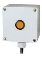
The **Exterior Time Lag Switches** are ideal for energy saving control of exterior heaters and exterior lighting. Also suitable for damp areas indoors. Pressing the button brings the connected load on. The load is then switched off automatically after the time lag has elapsed. The time lag can be set between 2-20 minutes. Illuminated touch area for easy location in the dark. Tough, hard wearing, with a IP66 rated polycarbonate moulding.
