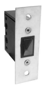
A **Door Switch** that enables you to turn a light on and off in a cupboard or room. When the door is closed on the switch the light would be turned off, as soon as the door is opened and the switch is released the light will turn on.
