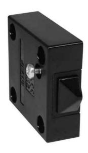
A **Door Switch** that enables you to turn a light on and off in a cupboard or room. When the door is closed on the switch the light would be turned off, as soon as the door is opened and the switch is released the light will turn on.
