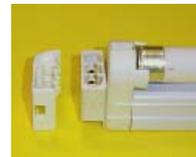
Socket end view with added protective cover removed
