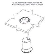
PIR ASSEMBLY PUSHES UP INTO HOLDER UNTIL IT GLICKS INTO POSITION FLUSH MOUNTED PIR
