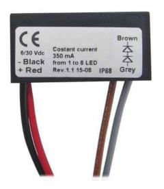
The **Wise Converter 3** is a power supply that is used to drive 350mA LEDs, but only requires an input of anything between 6 to 30V. This makes it ideal for use on boats, cars, caravans, or motorbikes where the supply is limited to low votlage, or for powering direct from a battery.
