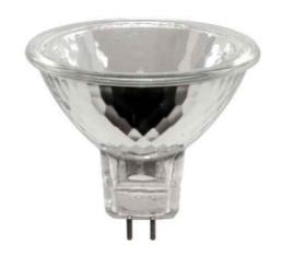
The Ultralife Halogen MR16 has a lifetime of 10,000hrs with a reflective aluminium coating applied to the inner surface of the lamp. This reflects heat and light away from the light fitting both protecting it and increasing its efficiency.
