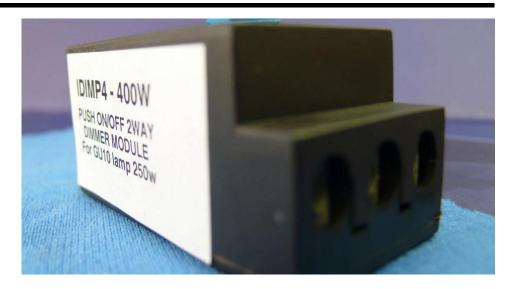
The **Resistive Load 2 Way Dimmer Module** allows you to custom make your own switches as they easily attach to standard manufactured wall plates. They are also used to replace faulty or broken modules in existing switches. If purchased for this purpose, please ensure that you select the correct wattage and check whether it is a an inductive or resistive load.
