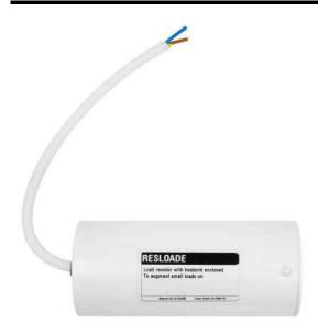
**Resload**, resistive load can be used to try to eliminate lamp instability and flicker when dimming non-resistive loads such as mains directly dimmable LED lamps, compact fluorescent lamps or dimmable transformers.
