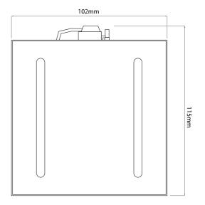
Section drawing for FRT100 Frame 15mm
