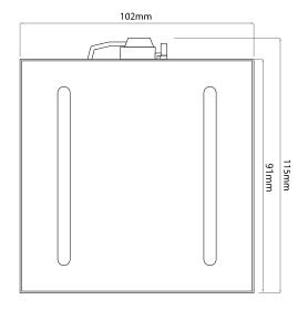
Section drawing for FRT100 Frame 15mm
