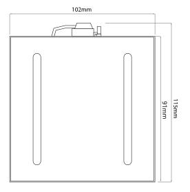
Section drawing for FRT100 Frame 15mm
