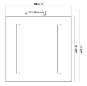
Section drawing for FRT100 Frame 15mm
