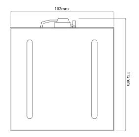
Section drawing for FRT100 Frame 15mm
