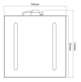
Section drawing for FRT200 Frame 15mm
