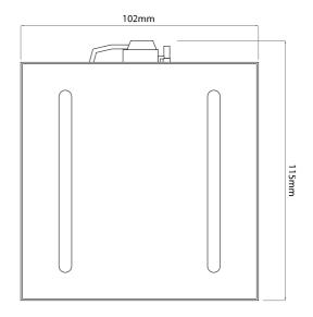
Section drawing for FRT200 Frame 15mm
