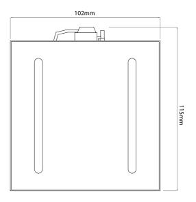
Section drawing for FRT200 Frame 15mm
