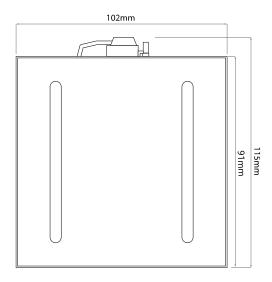
Section drawing for FRT200 Frame 15mm
