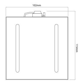
Section drawing for FRT200 Frame 15mm
