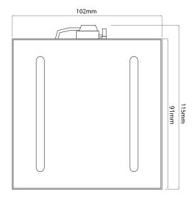
Section drawing for FRT200 Frame 15mm
