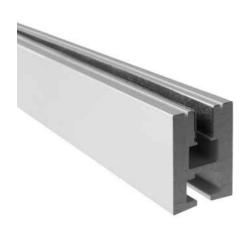
The **Glass Edge Surface Extrusion Profile** clamps onto a 6mm thick piece of glass (not included) which then projects the LED light through the side, illuminating any frosted pattern / text which has been imprinted onto the glass surface.
