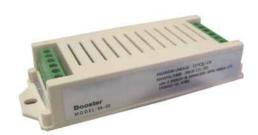
The **Feelux Booster** is used in conjunction with our *Seamless DimLine/DimSlim* range of products. Currently, if using a Feelux wired dimming switch or interface, a maximum of 10 fluorescent fittings can be used per channel. Use this product at the tenth fitting from the dimming switch or interface and the connecting capability extends 20 more pieces.
