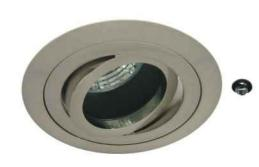
The **Black Baffle 50** is a fully adjustable 50mm downlight which has the added benefit over the *Rock 'n' Roll 35* of an integrated black baffle. This recesses the light source further into the downlight, absorbing light at wide angles to eliminate glare whilst also maintaining full light output. The inner ring can tilt to a maximum of 35Ű for precise beam placement.
