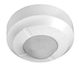
The **360° PIR Surface Mounted Occupancy Switch** utilises passive infrared technology to detect heat from a moving person. Upon detection, the attached lighting load will illuminate for a user-determined time period between five seconds and eighteen minutes. An integral daylight sensor ensures all day or night-only operation.
