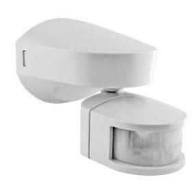
The **180° 2300W PIR Light Controller** can control loads reaching 2300 watts (max.) under a power source of 240V. It uses passive infrared technology to detect heat radiation of moving human bodies. Upon detection, the attached lighting load will illuminate for a user-determined period of time. An integral daylight sensor ensures all day or night-only operation.
