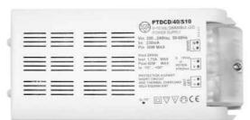
The **PTDCD40S10** has a dimmable independent constant voltage power supply. The 24V output voltage is PWM modulated (adjustable duty-cycle between 4% &100%) High efficiency and reduced weight and size.
